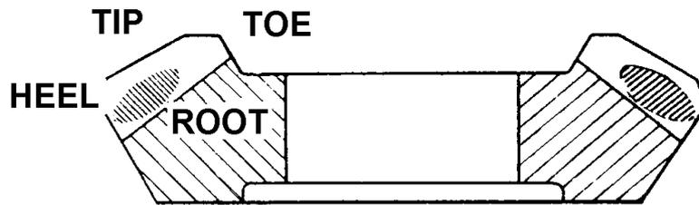
Contact markings closer to heel and root than factory markings
