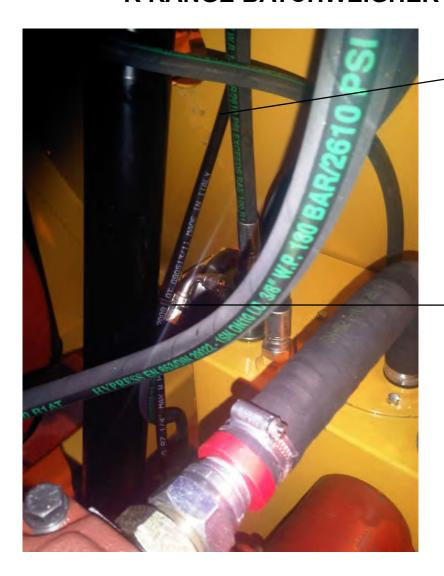
Secure to Mainframe using Hose Clip No 143200300, Setscrew No 16S05B, Washer Spring No 17S10 and Nut No 7S09.
