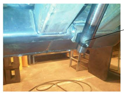
Striker Pin No 555109100, Secure to the Hopper Cradle with one 6S05E Setscrew and one 41S07 Spring Washer, sandwiching the Shim Pack between the Striker Pin and the Hopper Cradle. (See below) Lubricate the threads of 6S05E setscrew with copperslip before Inserting.
