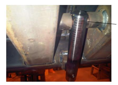
Install the Striker Pin to the underside of the Hopper Cradle. Lubricate the Retaining Pin and Bosses before inserting the Pin into the Hopper Cradle. Secure the Pin using the Grubscrew and tighten.
