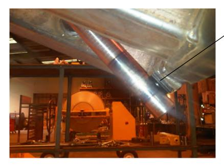
Insert 2 thick shims and 1 medium shim from Shim Pack Part No 555109200 between the Striker Pin and Hopper Cradle. (Part Nos 555109203 x 1 & 555109204 x 2) Sandwich the medium shim between the two thick shims to prevent distortion when the retaining setscrew 6S05E is tightened.
