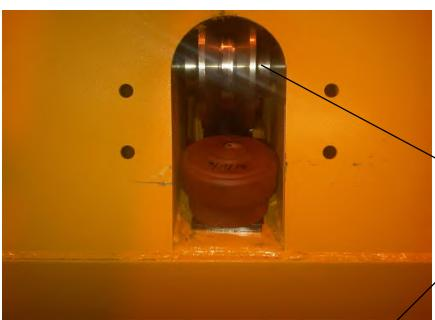
Carefully install the Bearings No 113149000 and Seals No 422702000 into the Striker Guide No 555108900.
