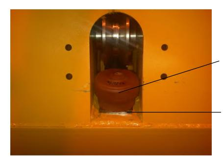
Load Cell installed in mainframe. When routing through interior of mainframe ensure the Capillary Hose is not "kinked or damaged or allowed to chaff on components or other hydraulic hoses.
