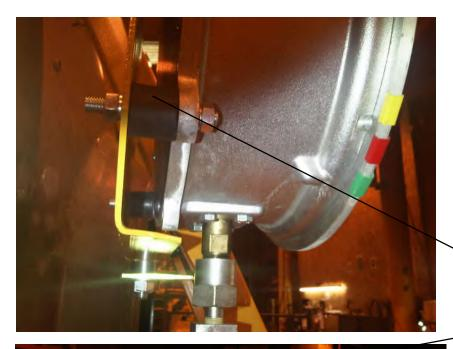
Assemble the Weighbatcher Gauge (Part No 555242414 on the 300R/400R & No 555242418 on the 500R) to the Retaining Brackets whilst the Gauge is resting on a suitable bench. Take care that the Capillary Hose between the Gauge and Loadcell is not "kinked" or damaged during this process. The four holes in the rear of the alloy body of the Gauge will require opening out with a suitably sized drill bit to allow fitment of the rubber Anti vibration mounts No 013203000.
