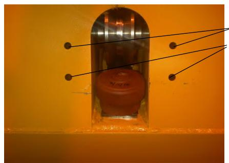
If installing a Batchweigher to an existing basic machine remove the two stop blocks No 555109600 from the face of the mainframe.
