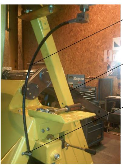
Note the long radius on the Capillary Hose to avoid "Kinking" or damage.
