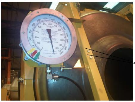
Weighbatcher Gauge installed on Mixer note long radius on Capillary Hose to Load Cell to avoid "Kinks"
