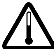
General hot surface warning
