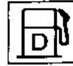
Diesel fuel fill
