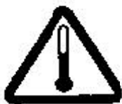
General hot surface warning
