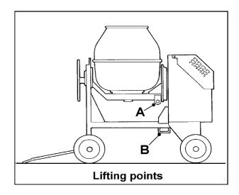
Spread the fork tines and carefully position the forks below the mainframe so that one tine enters and passes through the bracket 'B' below the mainframe, the other fork should be spread as wide as possible. Position the carriage as close as possible to the mixer and rest the mixer's drawbar on one of the fork tines to prevent it swinging freely.
