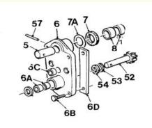
**Tilting Pinion Assembly for Handwheel** Complete castings assembly with pinion, stub pin and all bushes and bearings (fully lubricated).
