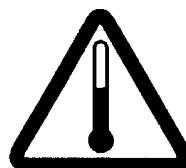
General hot surface warning
